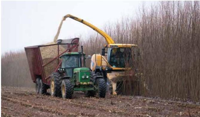
Harvesting willow biomass crops with a specially designed cutting head attached to a forage harvester. Photo courtesy of Tim Volk.
