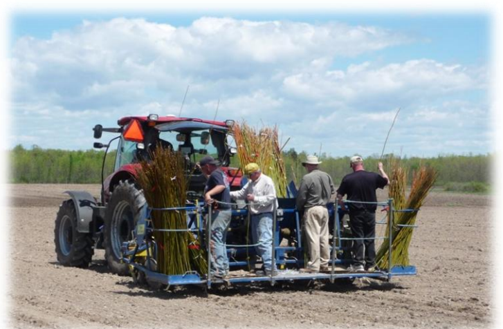
A tractor-mounted planter establishing willow in NY State
